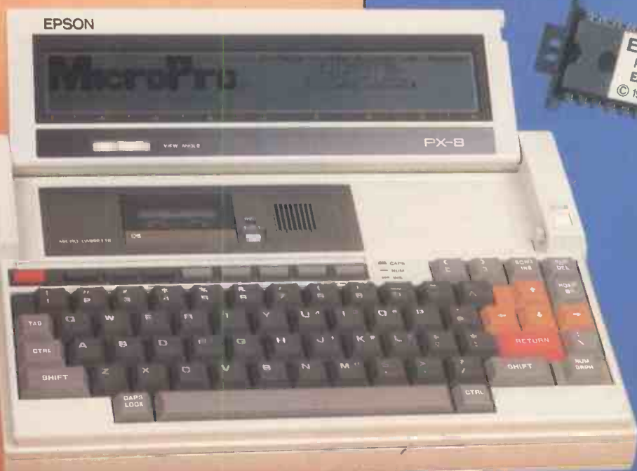
Below: The compact PX-8 runs CP/M software and offers WordStar on a ROM.
