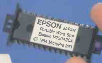
Below: The compact PX-8 runs CP/M software and offers WordStar on a ROM.
