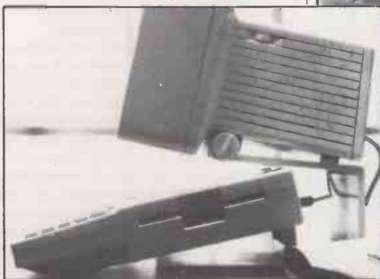
A half-height floppy drive is built into the side of the IIc. The monitor and mouse are optional.
