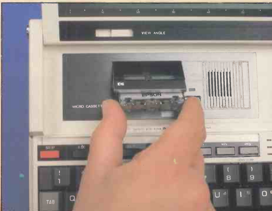
Above: The built-in microcassette drive can hold about 32K on each side of a cassette.
